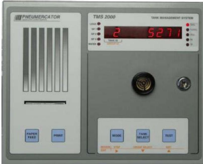
A front panel horn is provided to annunciate alarms as well as communications failures. When a leak or system failure occurs, the alarm will sound and the indicator lights and/or LED panel will identify the reason for the alarm.
